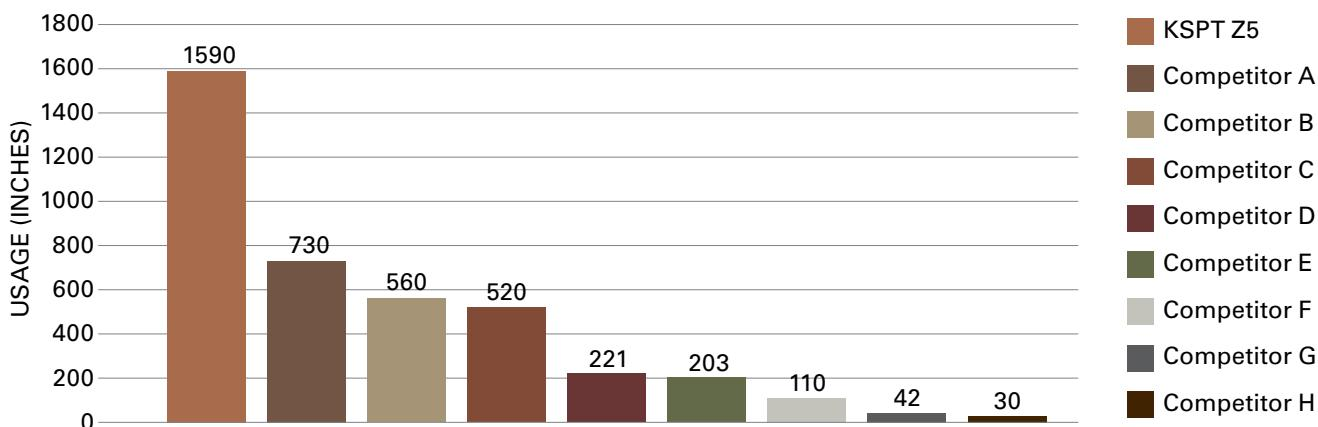
RESULTS IN STAINLESS STEEL 316 @ 160HB Z5CR 1/2" TESTED AT 2540 RPM X 31.7 IPM
