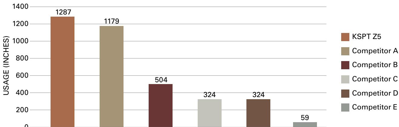
RESULTS IN TITANIUM 6AL4V @ 32HRC Z5CR 1/2" TESTED AT 1643 RPM X 16.4 IPM
