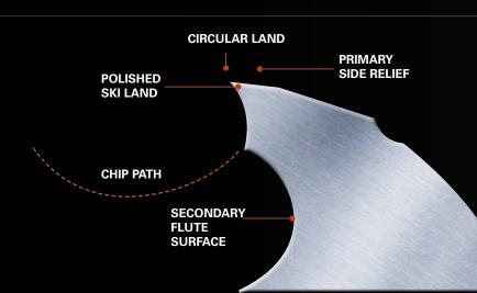
Tight control of the circular land width reduces edge aggressiveness, which allows for a wide variety of speed and feed rates. It also allows for milling into corners without chatter. Unique to the Ski-Carb is the primary-secondary flute wall construction, which reduces chip interference.
